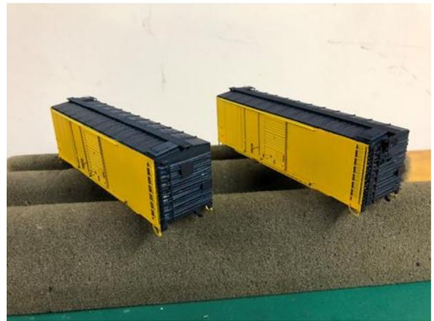
Fig. 11 I masked the sides and sprayed the darker color.
