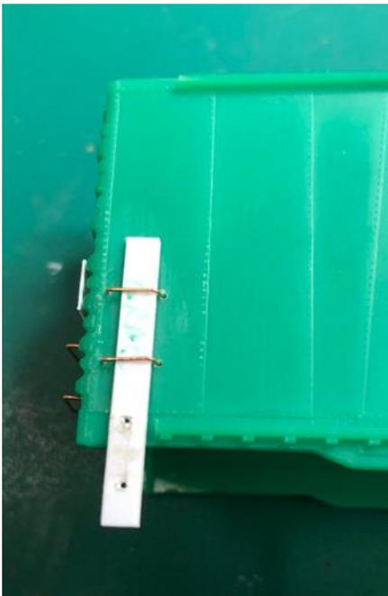
Fig. 7 Jig for uniform grab iron depth.
