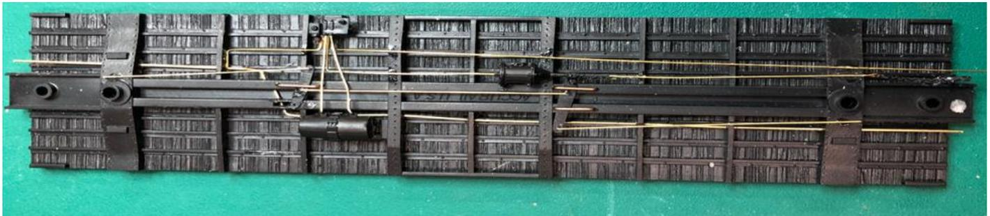
Fig. 4 Completed undercarriage AB brake parts with air lines.
